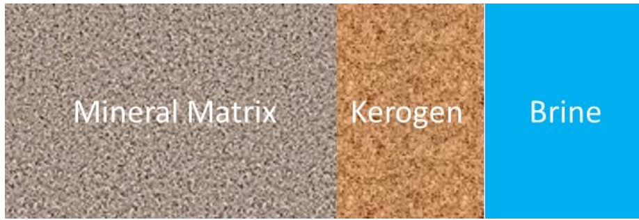
Fig. 2— A schematic representation of an immature organic shale source rock. The porosity is 100% water filled. Note that kerogen is not considered part of the porosity. The brine includes all water both clay-bound and free.
