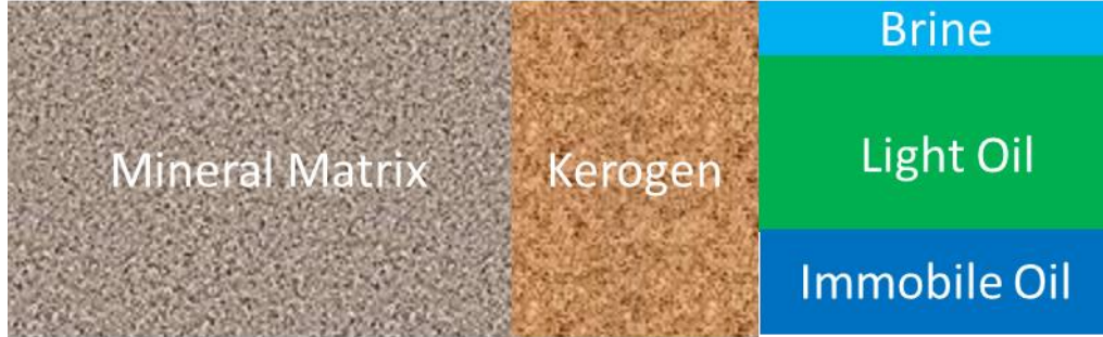
Fig. 3— A schematic representation of an organic shale tight oil reservoir. The three fluids that occupy the total porosity are brine, high-gravity producible oil, and bitumen and/or immobile oil.
